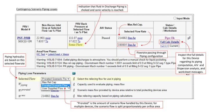
The term "Relief Flow" is replaced with "Selected Flow" to represent the flowrate that is selected by the user for the determination of the piping losses. These displayed piping losses can be calculated at three different selections; Maximum Relief Capacity (of that device), Prorated Scenario Flow, and a User Supplied Flow.
