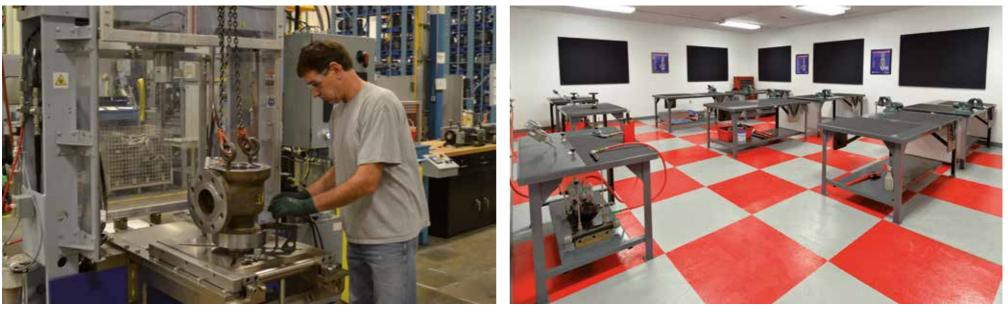
Ergonomically Designed Hydrostatic Testing Station (LEAN investment).
